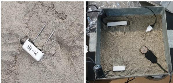
Figure 5: Installation of TERSO 10 during model build-up (left) and calibration for clean sand.
