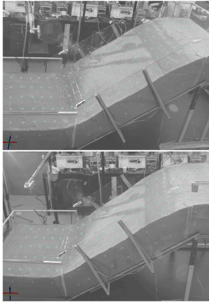
Figure 3: Left-camera (top) and right-camera (bottom) view of the model with monitored points (green dots) (from [2, 15]).
