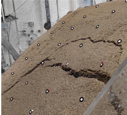
Figure 1: Pins with attached markers on the surface of the model.
