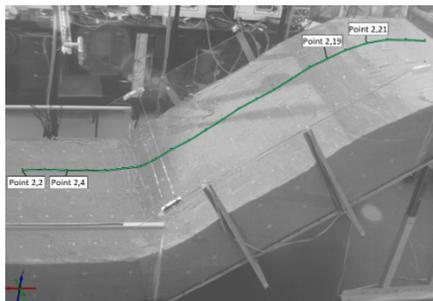
Figure 4: Longitudinal profile no. 2 in the reference stage and the location of the points used for the detailed analysis of the displacement evolution.
